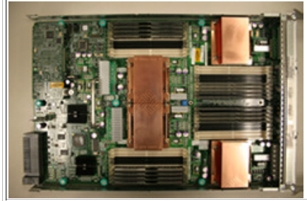
Figure 2. SunBlade x6420 motherboard.
